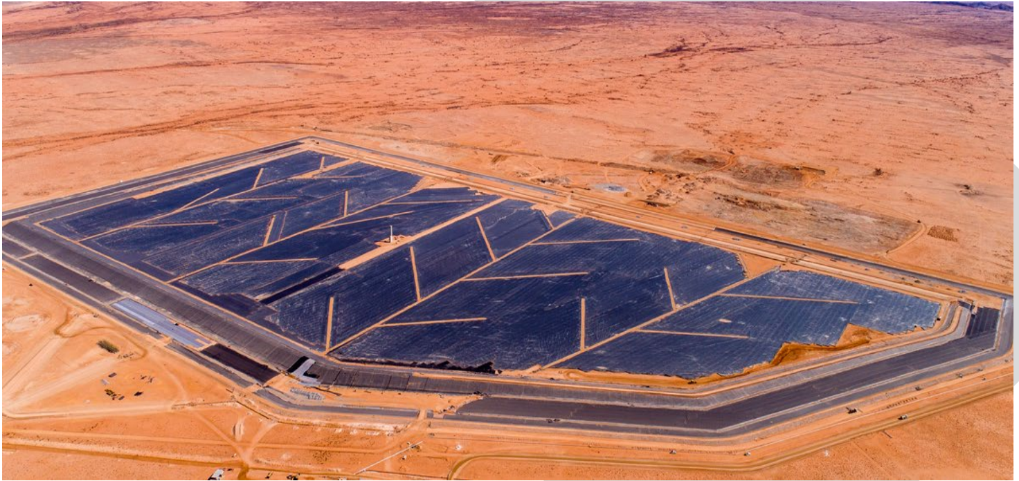
Tailings Storage Facility, Capacity: 30mil m 3 /12 years, Northern Cape
